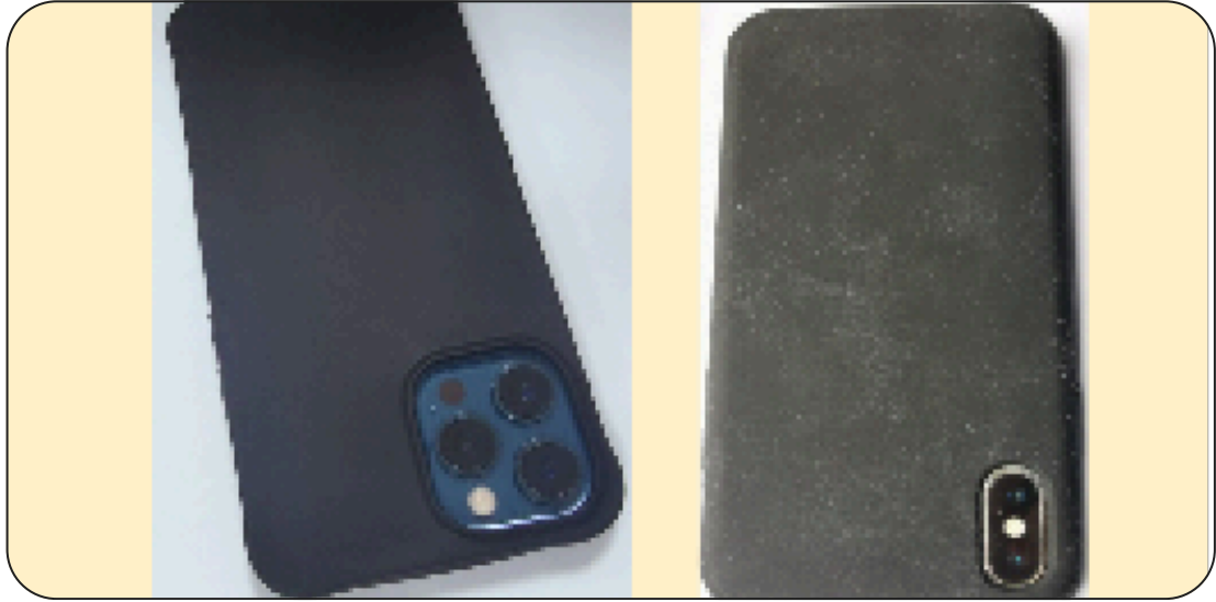
Outstanding stain resistance. Under the same one-day use conditions, the SkinTouch phone case (left) shows significantly better stain resistance than the silicone rubber phone case (right).
